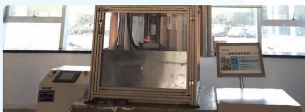
Hammer Dropping Impact System for Impact Resistance Test
