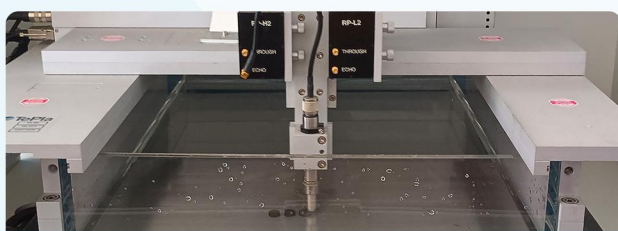
Internal Defect Inspection - Ultrasonic C-Scan
